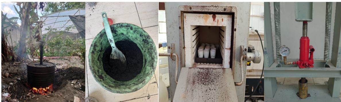
Figure 2. Manufacturing Process of Biobriquettes from Sugar Palm ( Arenga pinnata ) Waste
