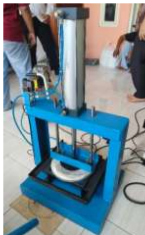
Figure 5. Automatic Pneumatic Molding Machine
