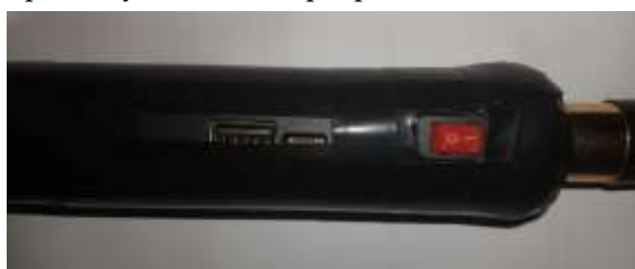
Figure 4. Rechargeable Battery Charging Port and On/Off Button of CHEMLIT
